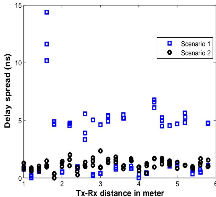
Figure 5. Delay spread in both scenarios.
