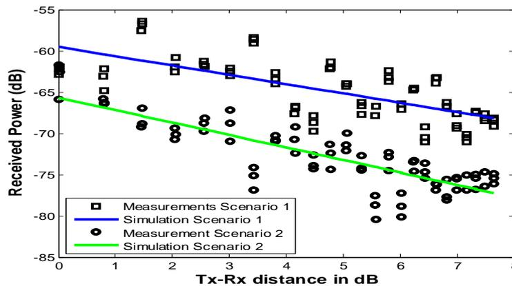
Figure 6. Path loss results in both scenarios.
