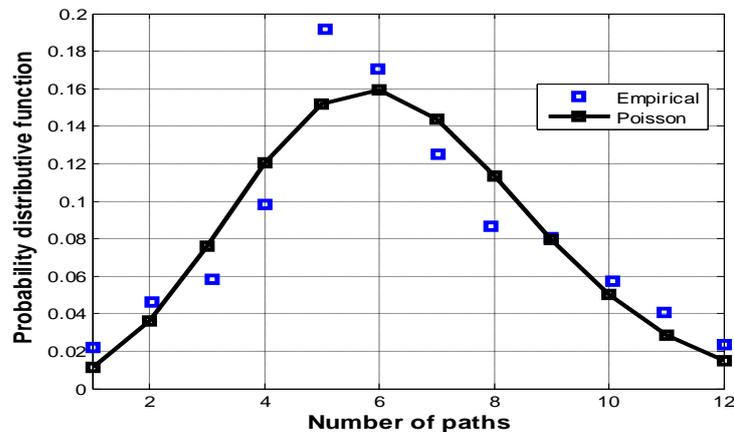
Figure 4. Probability distribution function of the number of paths of scenario 2.
