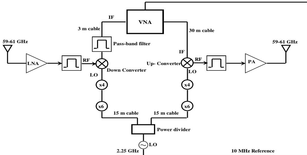
Fig.2 Measurement set-up
